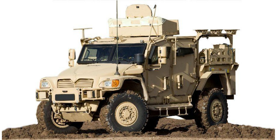
Husky Protected Support Vehicle Modified to Theatre Entry Standard
