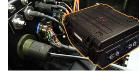
Application: Data Acquisition & Logging System
